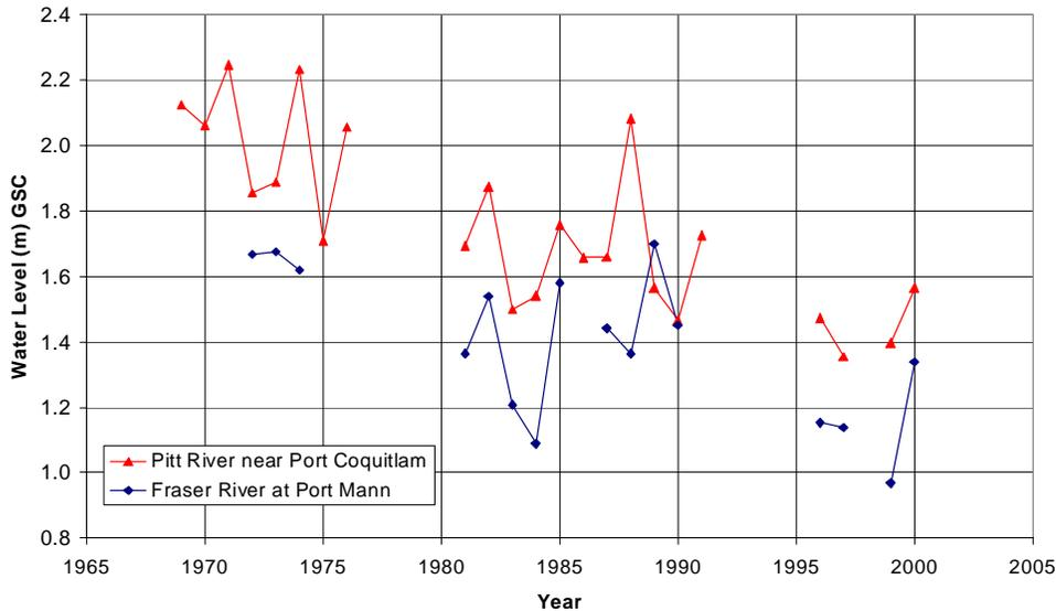
**Figure 4: Trends in Water Levels at a Constant Discharge and Tide Level**
