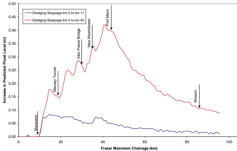
**Figure 5: Potential Effect of Curtailing Dredging Operations on 1894 Design Flood**
