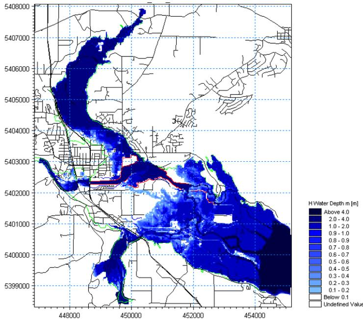
**FIGURE 2: Modelling Results of Channelized Flows and Overbank Spilling - Maximum Water Depths for 200-year Flood (freeboard not included)**
