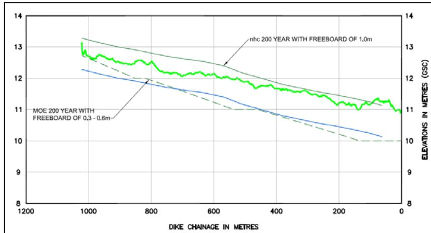
**FIGURE 3: Dike and flood profiles (with and without freeboard) for 200-year flood with all existing dikes confining the flow.**
